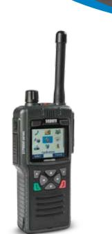
The STP9100 hand-portable combines extreme ruggedness with powerful audio and RF. Waterproof, submersible, dust-proof and marine-hardened, the IP67-rated STP9100 provides the latest smart technology to users who need a high specification, reliable radio, but prefer a more streamlined user interface.
